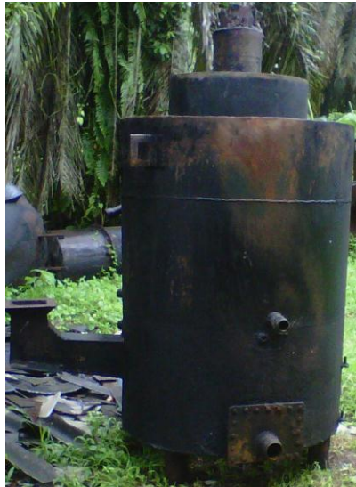
Figure 11d Crude oil clarifier
